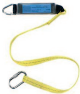
RGL1 EN354 and EN355 44kN polyester webbing Length 1.3m and 1.8m Shock absorber pack Maximum arrest force <6kN
