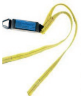
RGL3 EN354 and EN355 Twin leg lanyard 44kN polyester webbing Length 1.3m and 1.8m Shock absorber pack Maximum arrest force <6kN
